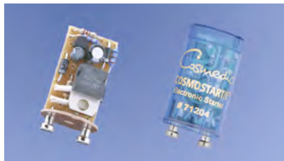
electronic starter without and with polycarbonate cover
